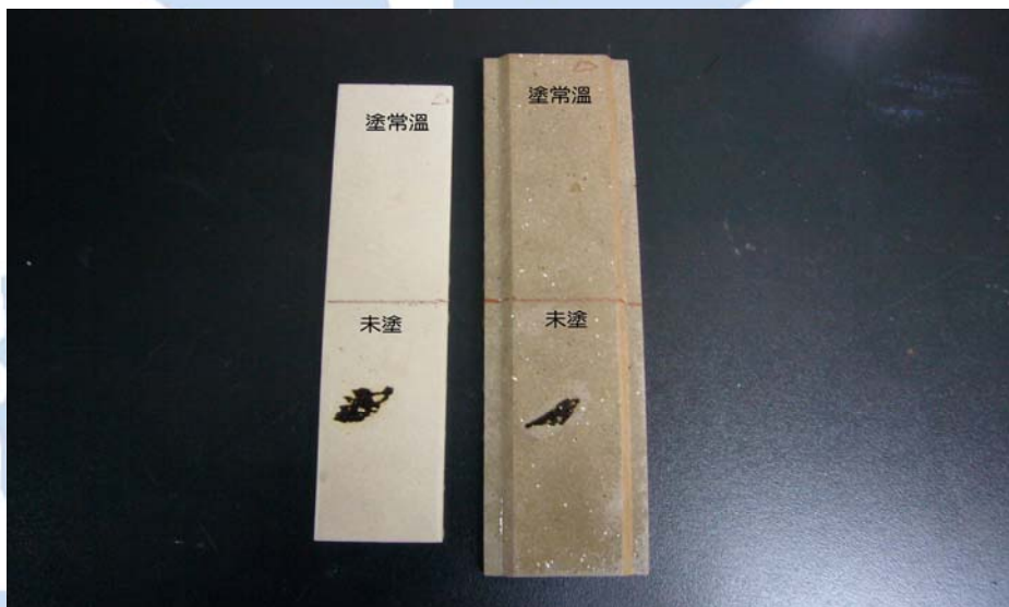
Picture: It can clean away greasiness on white exterior wall with the spreaded medicament by water flushing after 30 seconds,
